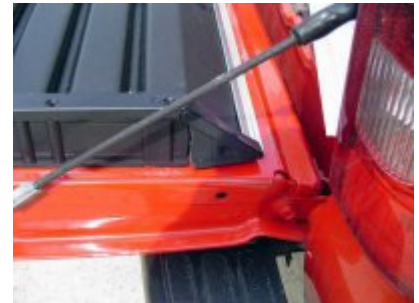
During shipping, a small corner of the X-treme gate was damaged.
