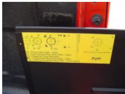
A template is provided on both side panels for location of the latch and retaining post mounts.
