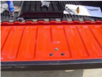
Bedliner panel was removed to install the X-treme-Gate.
